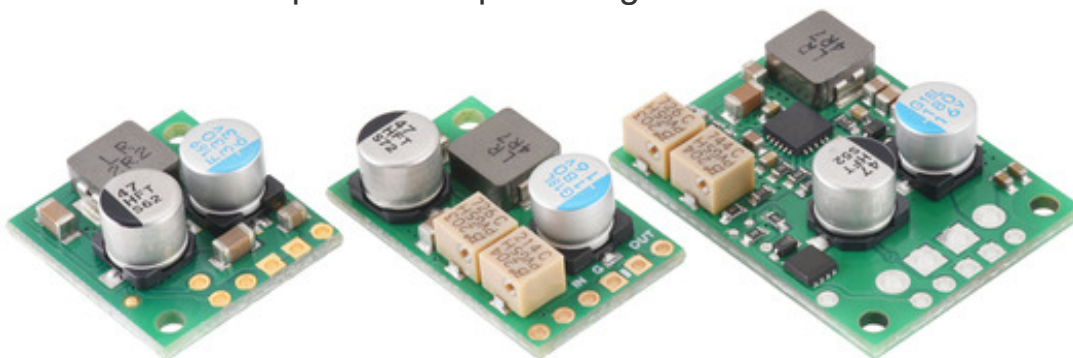
D30V3x line of step-down voltage regulators. From left to right: D30V30Fx, D30V30MASx, D30V33MASx.
